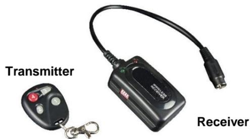
The receiver connects to the remote control socket on the machine and has a magnet on the back for attachment. The receiver's red LED indicates the machine is heating; when it goes off, the machine is ready to use.
