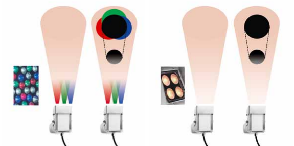
Single-color LEDs Different single-color pixels result in color separation near the fixture and shadows
