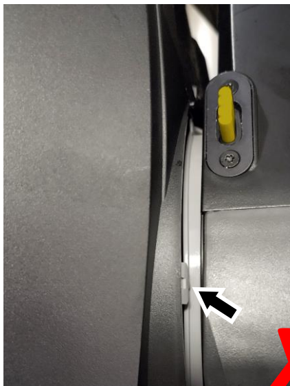
Incorrect – tab outside head cover
