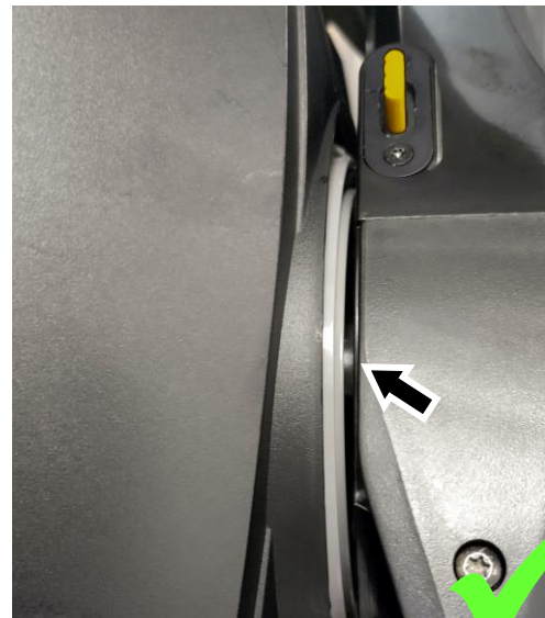
Correct – tab inside head cover
