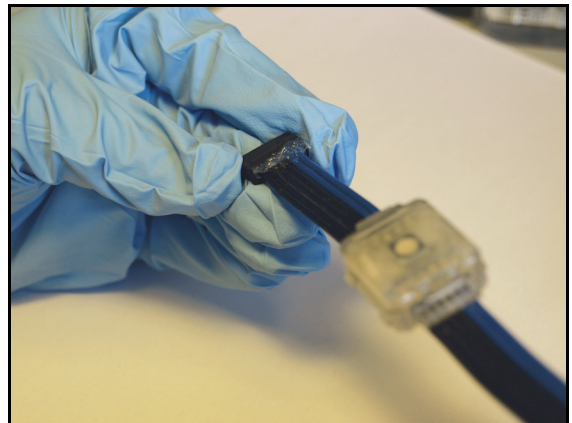
Figure 3. Applying sealant and installing a cap
