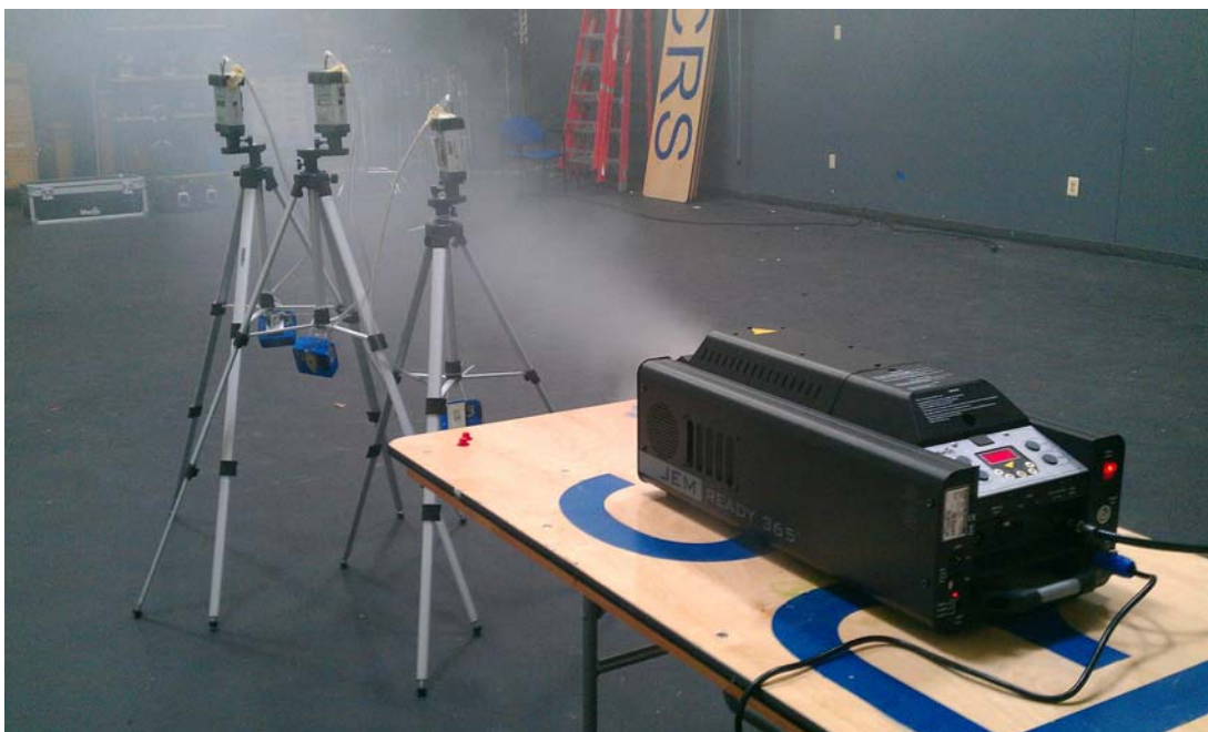
Figure 1. Configuration for calibration factor procedure, consisting of the tripod assemblies with sampling pumps, OVS tubes for sampling glycols, and aerosol monitors.
