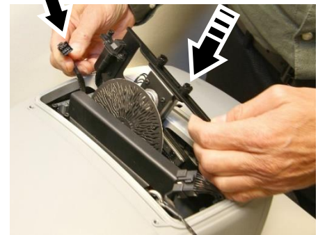
Installing an animation wheel module
