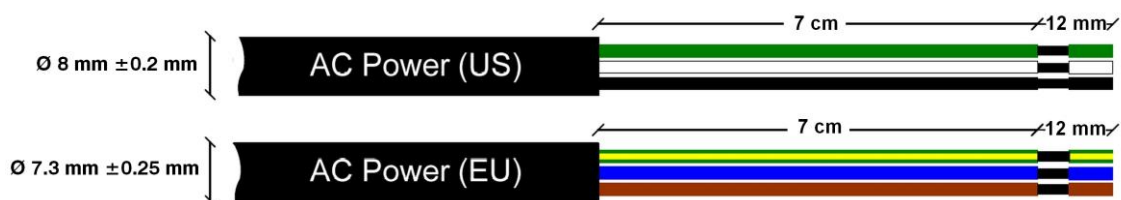
AC power cable details
