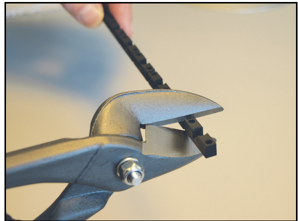
Figure 3. Cutting mounting ribs
