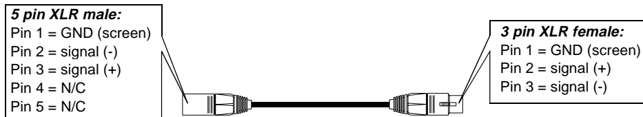
The above figure shows the cable to connect from 5-pin DMX output to 3-pin input on Martin fixture (P/N 309162).
