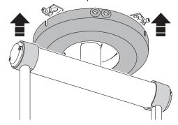
8 Using the 3 mm Allen wrench, tighten the three Allen screws that hold the cover in position.
