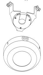
2 Using the 3 mm Allen wrench to loose the two locking screws, remove the slotted section of the J-Box.
