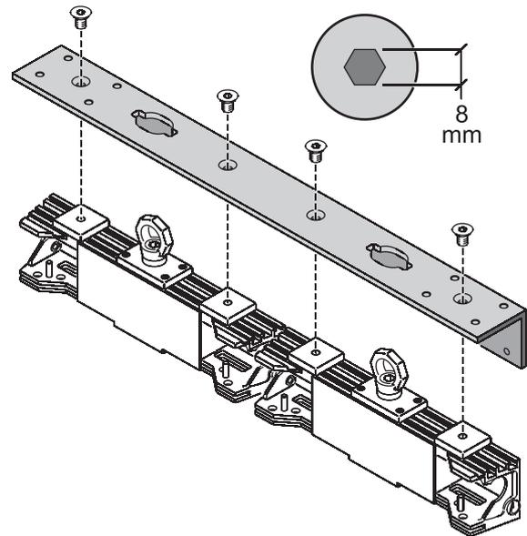
Figure 5: Header Connection Bracket (Double Header illustrated)
