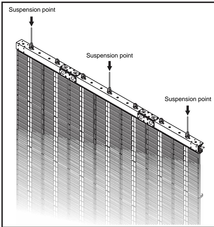
Figure 7: Installation 7 panels wide
