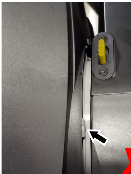
Incorrect – tab outside head cover
