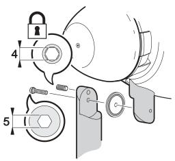
2 Attach the base of the arm to the required surface using M6 mounting hardware that is appropriate to the mounting surface and to the weight of the fixture.
