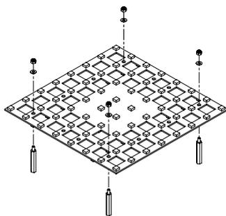
The VC-Grid can be fastened to a surface or structure using pillar bolts through any of the twelve mounting holes
