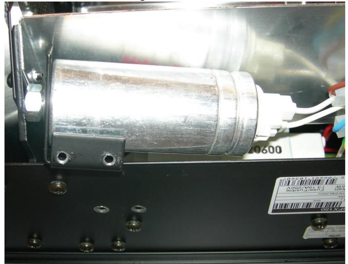
7. Fasten the mounting bracket to the casing.
