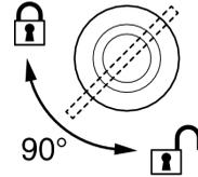
5. Working from a stable platform, hang the fixture vertically on the truss and fasten the rigging clamp onto the truss.
