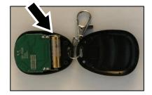
2. Open the remote and remove the white insulating tab (arrowed) from the end of the battery. Check that the battery is installed correctly and makes good contact with the battery terminals.
