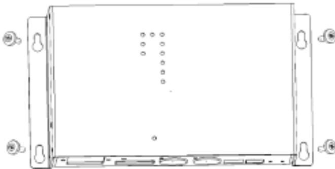
When mounting the device on the wall, ensure appropriate fastening. The device must be fastened so it can carry 5 times its own weight. Make sure that the device is only mounted in the orientation illustrated above.
