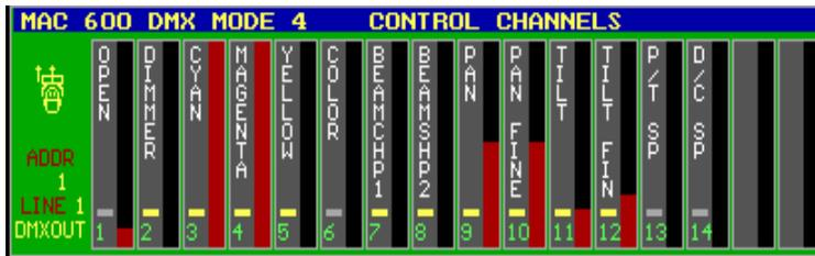
A channel that can fade is marked with a yellow box. A bump channel has a gray box.
