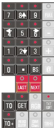
**In fixture mode [Adjust fixture control channels] [TO] [memory-number on keypad] [RET]**
