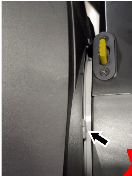
Incorrect – tab outside head cover
