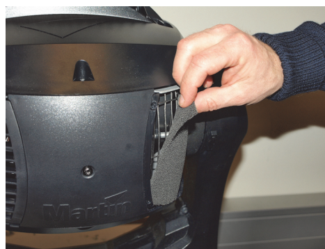
Figure 9: Removing head air filters
